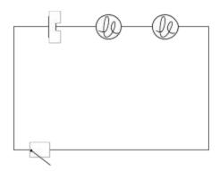
The voltage in this cell is shared by the two light bulbs, which causes the second bulb to be dimmer than the first.
