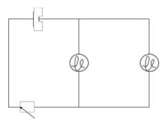
The voltage in this cell is shared equally by the two light bulbs. The bulbs will burn equally bright.
