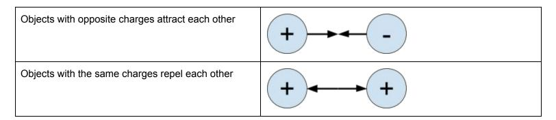
**Static electricity** occurs when two objects with opposite electrical charges come close enough to each other to allow electrons to move from the negatively charged object to the positively charged one. This electron movement is the cause of the shock a person felt or the zap heard or spark seen as the charged objects return to a neutral condition. A lightning flash is a very large discharge of static electricity.
