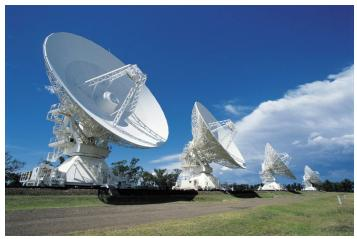
An advantage of radio telescope is that they use radio waves not visible light waves. Radio waves are not as easily distorted as light waves, and they are detectable at any time of day. Radio waves can detect objects that do not emit visible light. These telescopes can also be combined in **radio interferometry** to produce high resolution images. A group of many telescopes are called an **array**.
